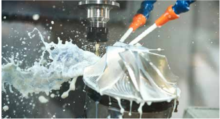
A chip-away process a milling machine cutting the block material
