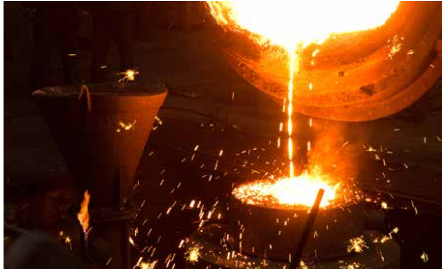
Melted material is being poured into the shaping mold in the casting process
