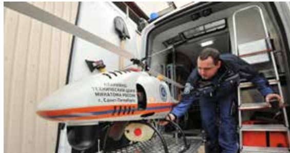
Preparation of an unmanned helicopter to a two-hour flight in the area of radiation accident radiation measurement, photography and videograph
